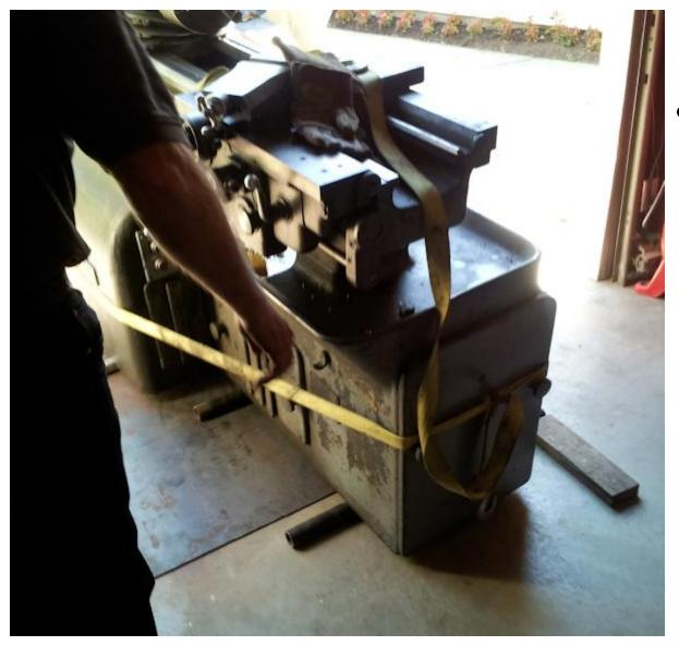
After trailer tips, lathe moves without need for strap puller
