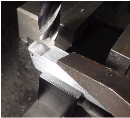
6. Front surface milled with the top of the fixture canted up 5°.
