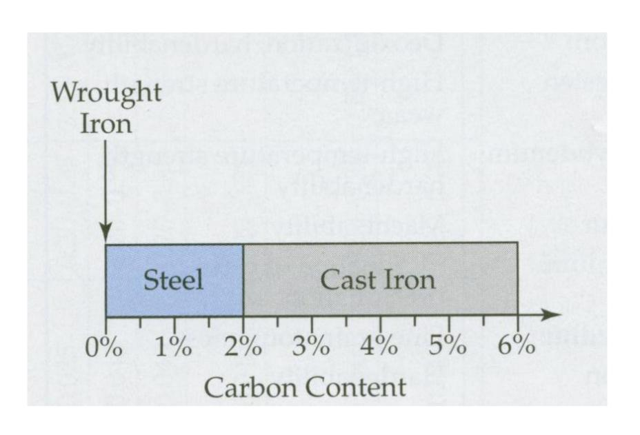
Since we are not interested in working with molten steel or cast iron for purposes of this talk, we will limit our attention to the lower left portion of the phase diagram.
