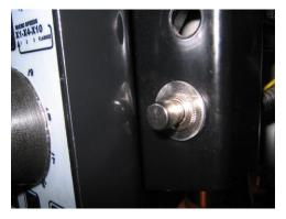
PROJECT ELEVEN – I swap out the switch for an unlighted heavy-duty push on/off button. This one works fine, except that the hole for the old switch is much larger than the neck of the new switch. No problem, I'll just make adapter pieces on the lathe, which I do. Switch ready. Block ready. G-code ready. Time to start...
