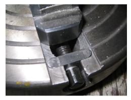
eccentric. I put the block back into the chuck and tightened three of the jaws, feeling really proud I had made such a neat fix. But the fourth jaw would not tighten? Now what? I took the mechanism apart and saw that one of the adjustment screws had stripped out. Arrgh! Now I have to do...
