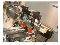
John talked about how he used his mill - lathe to build target rifle stocks employing stainless steel bedding blocks. The custom parts
