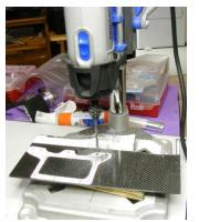
The next step is to cut out the outline on the glued pattern. John starts by cutting the straight lines with a <u>Dremel 4000</u> and a cutoff wheel. He then uses a drum sander on the Dremel to cut the contours and clean up the final shape.
