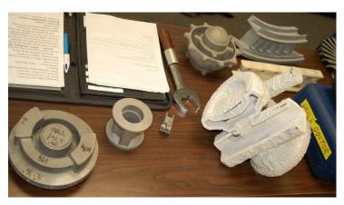
The pattern produced to form the mold will be larger than the final part, due to shrinkage of about 0.020 per inch. The exact shrinkage varies with different metals and with part geometry.
