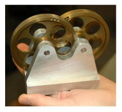
Dick Kostelnicek - balanced a motor shaft using a fixture he built that used very small ball bearings. He said that it was important to use dynamic balancing instead of just static balancing, which can do more damage to a long-wide device than doing nothing at all.
