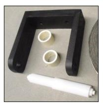
An abrasive shop roll is difficult to keep tightly wrapped around its spool when placed loose on a shelf or in a drawer. Here's a simple wood fixture that keeps these rolls in one location and ready for immediate use. It uses a spring-loaded toilet paper roller and
