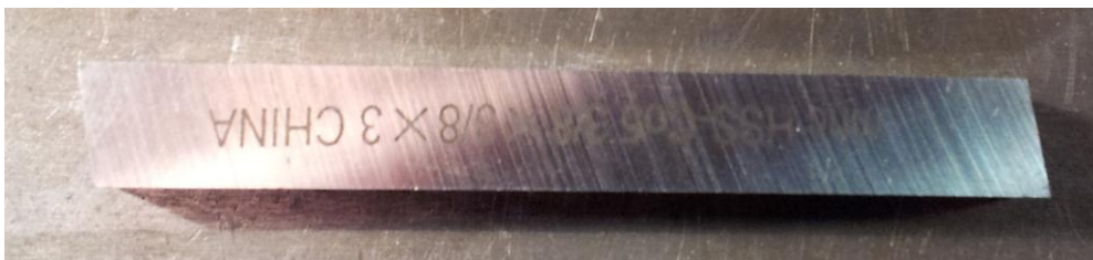
Slight Bevel on End of Tool Steel
