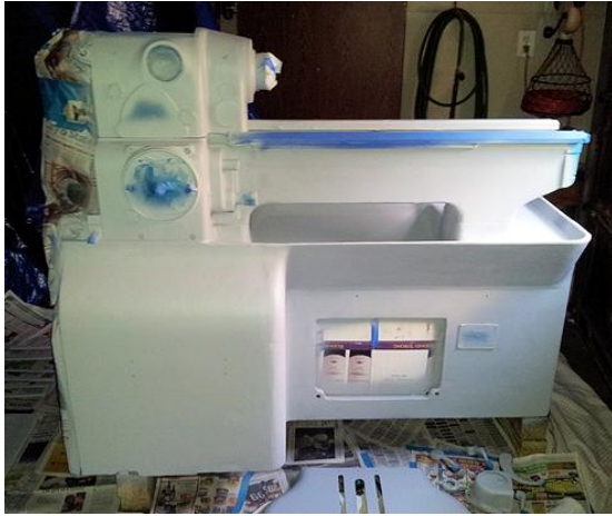
Lathe after taping and one coat of prime
