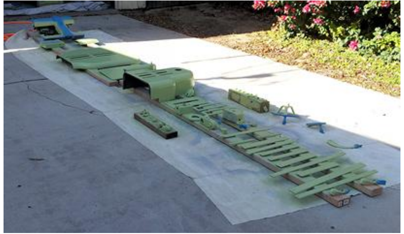
All the miscellaneous parts after one top coat
