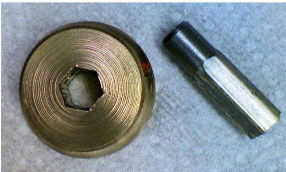
I had to replace a broken knob from a heat selector switch on a wire feed welding machine. The switch shaft was hexagonal in shape and about 11/32-inch across the flats. I made a replacement knob from brass and swaged the hex hole in its center.
