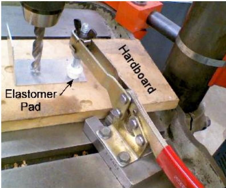
A horizontal toggle clamp makes for a handy method of holding down sheet material being drilled in a drill press. The alternative is to hold the sheet by hand or pliers, risk having the work get caught by the drill bit as it breaks through, and having it rotate and slice into your hand.
