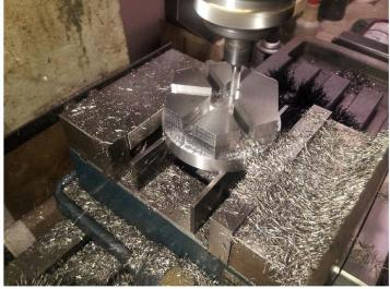
Cutting Slots w/High-Speed CNC Toolpath
