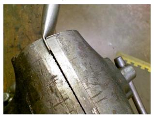
I made a strut from ½-inch **EMT** conduit (**Electrical Mechanical Tubing**) that is available at my local home improvement store. I squeezed the ends flat in a vise (left photo), and then, bent them to the proper angle.
