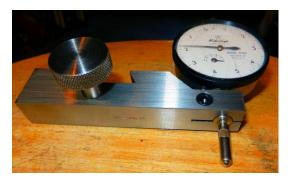
Here's the new design. The drawing is at the end of this article. I think that the new *design* (left photo) addresses the drawbacks of the first design (above right photo). It's easy to convert it to be used on the edge or the face of the stock in the lathe. The knurled screw was made such that a larger section of the shaft bottoms out on the top of the holder at the correct height to put the gauge at the center line of the lathe.
