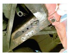
The hollow frame tubes have a ¾-inch wide oblong drain hole (above photo) that allows ventilation, and thereby, prevents moisture from rusting the inside of the tubes. I couldn't use a wrench to hold the 7/16-inch nuts inside the frame tubes. So, I fashioned a rectangular bar with two side-by-side 7/16-inch tapped holes. I welded a 1/16-inch gas
