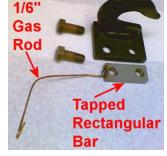
wedding rod to the bar in order to fish it inside the frame tube through
