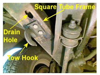
I wanted to attach two tow hooks (left photo) to the square tubular frame members on the undercarriage of a vintage 1964-½ Ford Mustang automobile. The two parallel frame members, running between the front bumper and the mid section of the vehicle, are made up from bent sheet metal that is welded into 4-inch square tubes. I didn't want to pass the bolts completely through the tubing since tightening the bolts could crush them and prevent firm attachment of the hooks.
