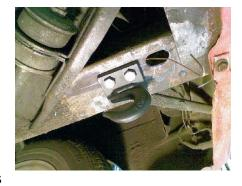
tightened, its neighboring bolt prevented reactive rotation of the bar inside the frame tube.
