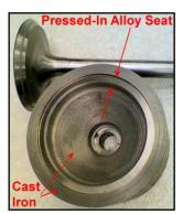
Recently, I learned about heat shrinking a steel part by welding. At the same time, I was interested in replacing an interference fit alloy valve seat in the cast iron cylinder head for an IC engine. The left photo shows a round 1.7550-inch OD alloy valve seat that was pressed into the cavity of a mock-up of a cast iron intake valve port (see right drawing). The hoop shaped seat is 0.2160-inch thick, 1.5000-inch ID and was pressed into the head with a 5
