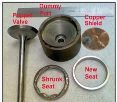
After inserting the stem end of the poppet valve through the back side of the valve guide hole (see upper right drawing), the copper disk was pushed out from the engine head. The copper disk, which was trapped behind the weld bead, pushed the heat shrunk seat out from its cavity. The measured OD of the seat after shrinking was 1.7432-inch, for about 12 thousandth inch shrinkage or 0.7% from the original 5 thousandth inch interference fit.
