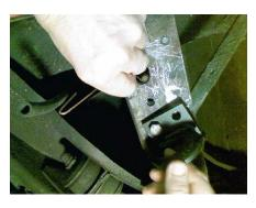
I screwed two bolts into the internally placed tapped bar and tightened them using much more torque than would have been possible if the bolts were 5-inches long and passed completely through the square frame tubes. There was no need to hold the threaded bar to prevent it from rotating, as would be the case for a nut. As each bolt was
