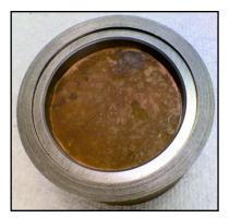
Prior to laying down a bead with a MIG welding gun, I placed a 0.03-inch thick copper shield disk inside the seat (left photo). The disk prevents the inadvertent welding of the seat to the cast iron head. Additionally, it prevents weld splatter from entering the head's port. The weld bead, around the inside of the seat, can be seen in the right photo.
