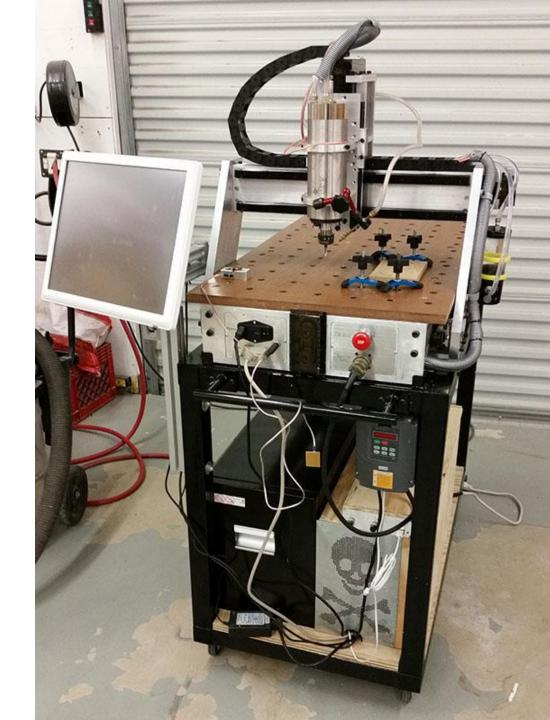
The machine I brought today is a modified Chinese 2030 type machine. This machine was design specifically for milling printed circuit boards and other thin flat work.
