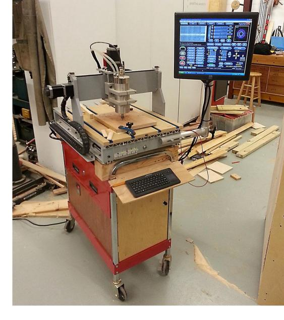
Although the 6040 machine functioned well, I decided to build a larger machine from scratch. The plan was for a machine designed mostly for woodworking, but capable for fine work such as milling printed circuit boards.
