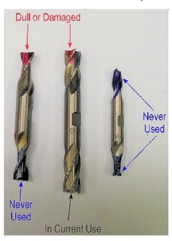
Grabbing an end mill and immediately knowing if it has been used or damaged requires somewhat more sophistication than the usual visual or tactical inspection. In fact a slight encounter of a finger with a very sharp new end mill can draw blood and send you scurrying to the first aid kit. You have a kit in your shop, don't you?
