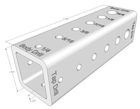
Here is a simple to make fixture that helps keep drilled and tapped holes perpendicular to a metal surface. It's made from a length of 2-inch square ¼-inch wall tubing
