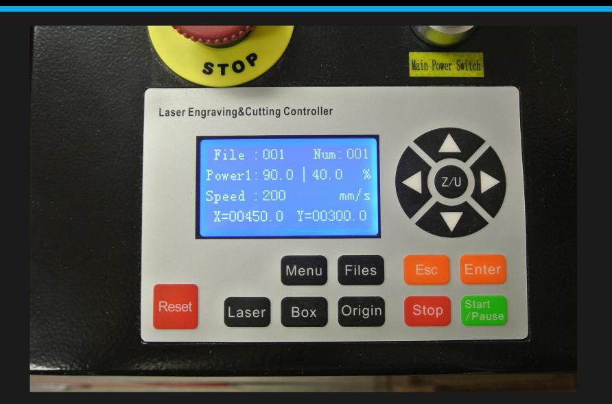
The front panel controls allow the user to set the origin of the job. Pressing the Box button causes the machine to trace the outer extents of the job, with out the laser on. This allows you to check and make sure the job will be cut where you expect it to be. The Start button starts the job. Never leave the laser while a job is in progress. The danger of fire is always present.
