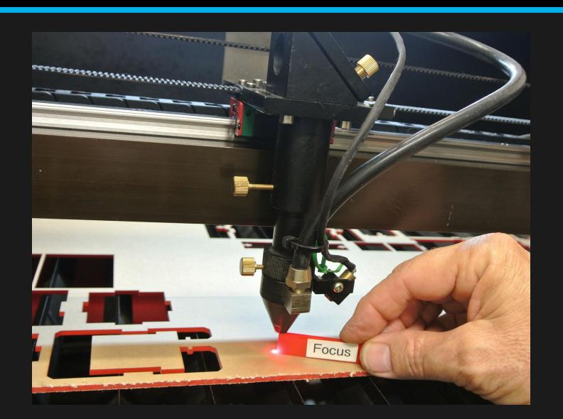
Before use, the laser must be focused. In improper focus can cause a fire, so this step is very important.
