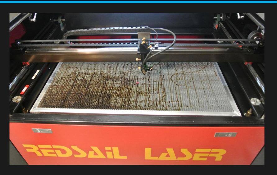
For small pieces the honeycomb bed works best. The bed is made of steel which allows the use of magnets to hold light materials in place.
