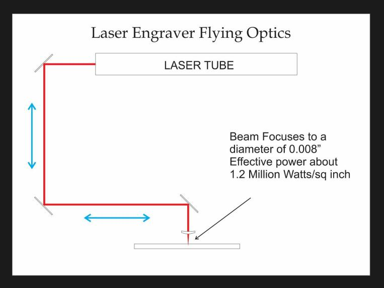
The laser tube and first mirror are stationary. The second mirror rides on the gantry, and the third mirror rides on the cutting head. Although the distance the beam travels changes with the position of the head, it makes little difference. The beam is focused to a tiny dot by a lens in the cutting head. Compressed air is fed into the nozzle chamber to cool the lens, keep smoke from getting on it, and clear the smoke from the workpiece.
