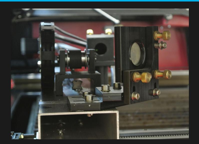
This is a view looking from the left side of the machine. The second mirror is in the foreground, the third mirror is located on top of the cutter head. Periodically, cleaning and alignment of the mirrors is done to retain best performance.
