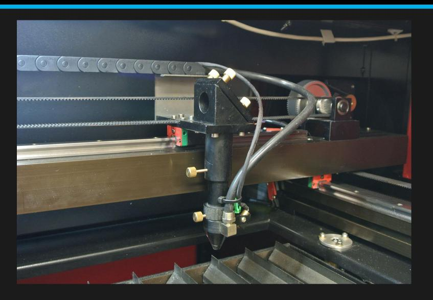
This is the cutting head assembly. It is driven on the X axis of the machine riding on top of the gantry. The mirror at the top of the assembly reflects the laser power down through the lens. The lens is located just above the nose cone. There is a compressed air line feeding air into the nose cone. This helps cool the lens and keep it clear of smoke.
