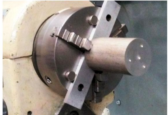
Securing shim behind part in chuck
