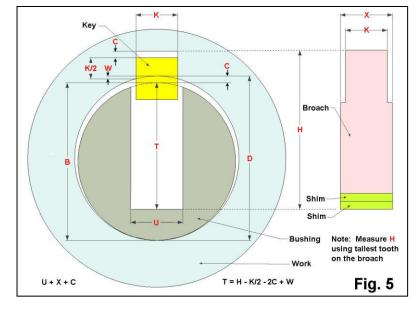
The three clearances **C** (Fig. 5) are all the same and are taken as 2.4% of **K**, the square key size. You, however, may choose **C** to suit your preference. The chord thickness **W** (Fig. 5) is determined where the key's half height touches the shaft's outer surface. It is calculated as:
