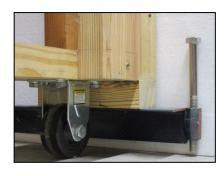
Three inch wheels, two fixed and two that can swivel, were screwed to the bottom framework. I then screwed a 2x2x 1/8 angle to the bottom of each end of the table. Blocks were added beforehand to elevate the angle to clear the wheels. Welded to each end of the two 2x2x 1/8 angles is a ½-13x 1 3/4 threaded coupling. Through the
