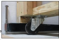
couplings are ½ x 6 inch long bolts that serve as leveling feet. Finished height of table is 42 3/8 inches. I used a bead of caulking to secure an aluminum (6061) top to the table. The aluminum top prevents cutting fluid and other liquids from penetrating the plywood table top.
