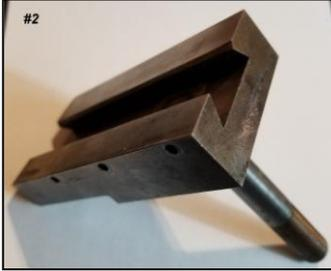
A participant has a 9x20 hobby bench lathe that suffers from a lack of rigidity. The lack of rigidity stems from the compound slide which lacks a locking screw. See photo at right.
