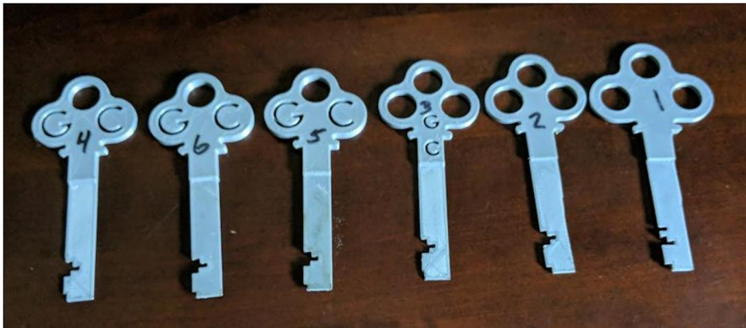
I ended up printing 6 keys. Starting with key 4, I could open the lock. From this point, I was able to make minor (~ 0.010") tweaks to the model to make the key fit better and reduce the play. The last key opened the lock smoothly. Time to make it in brass!
