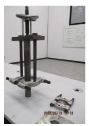
John Cooper showed a tool he made to remove a bearing from a 14 inch long shaft. See photo at left. Also, Cooper showed an example of holes drilled in angle iron with an annular cutter acquired recently. See photo at
