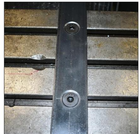
*Rich Pichler* exhibited stainless steel Rivet Nuts he used to repair a wheel mount on a utility cart. See photos below.
