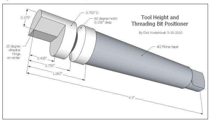
The positioning tool, shown below, can ensure both accurate height and bit alignment when it is placed in the lathe's tailstock ram. It is machined from a commercially available 2MT to 3JT drill chuck arbor.
