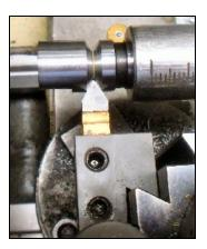
Using a dihedral hinge to gauge height and a V-notch to set bit alignment are certainly not a new concepts. What I've tried to do here is to combine setting height and bit alignment into a single tool that slips into the tailstock ram's socket.
